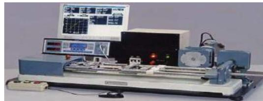
Figure 2: Tensometer
